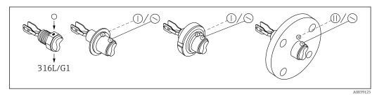
€ 23 Markings for aligning the tuning fork
