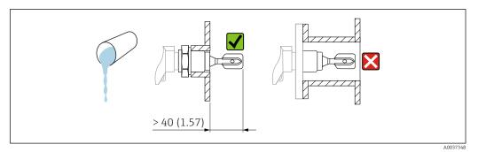
$\blacksquare$  20 Installation example for a highly viscous liquid. Unit of measurement mm (in)
