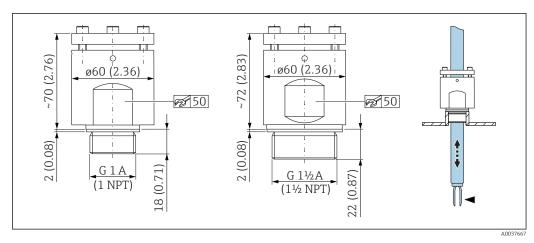
■ 66 High pressure sliding sleeves. Unit of measurement mm (in)
