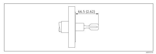
$\blacksquare$  51 Example with flange. Unit of measurement mm (in)
