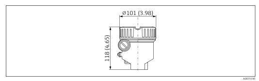
■ 34 Single-chamber housing, 316L, cast for Ex d/XP area; Product Configurator: order code for "Housing; material", option C. Unit of measurement mm (in)
