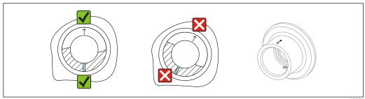
Weld-in adapter with leakage hole
