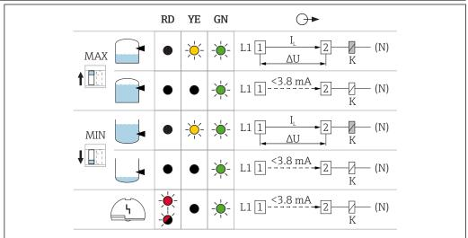
$\blacksquare$  3 Behavior of switch output and signaling, electronic insert FEL61
