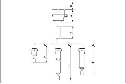
Components for determining the height of the device
