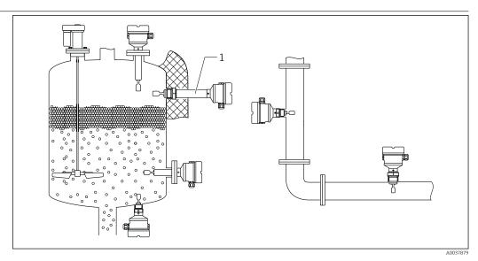
■ 18 Installation in any position in a vessel, pipe or tank
