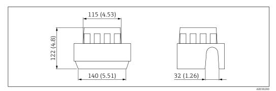
$\blacksquare$  60 Weather protection cover for single-compartment housing, metal. Unit of measurement mm (in)
