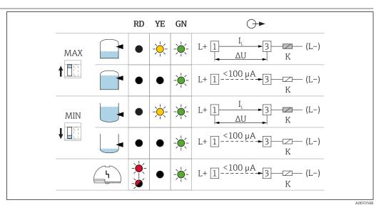
$\blacksquare$  5 Behavior of switch output and signaling, electronic insert FEL62
