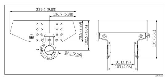
$\blacksquare$  59 Weather protection cover for dual-compartment housing, aluminum. Unit of measurement mm (in)
