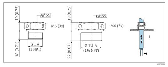
■ 65 Sliding sleeves for unpressurized operation. Unit of measurement mm (in)
