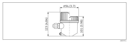
Single-chamber housing, plastic; Product Configurator: order code for "Housing; material", option A. Unit of measurement mm (in)
