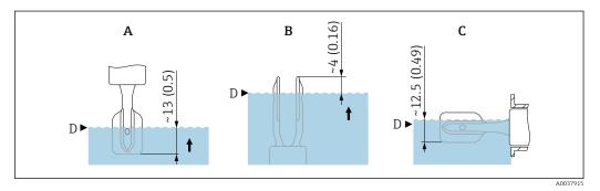
■ 16 Typical switch points. Unit of measurement mm (in)
