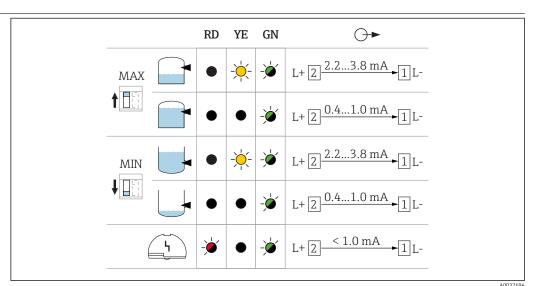
$\blacksquare$  13 Behavior of switch output and signaling, electronic insert FEL68
