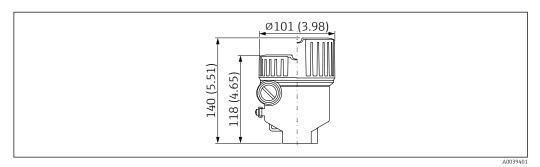
Single-chamber housing, aluminum for Ex d/XP approval; Product Configurator: order code for "Housing; material", option B. Unit of measurement mm (in)
