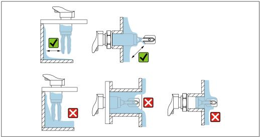
$lap{1}{2}$  21 Installation examples for a highly viscous process medium
