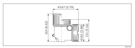
■ 35 Dual-chamber housing, L-shaped, aluminum for Ex d/XP area; Product Configurator: order code for "Housing; material", option M. Unit of measurement mm (in)
