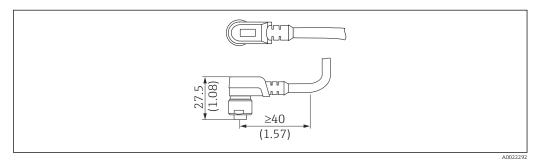
■ 62 Plug-in jack M12 IP67. Unit of measurement mm (in)
