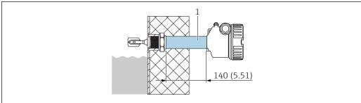
**■** 36 Temperature spacer, pressure-tight feedthrough (1). Unit of measurement mm (in)
