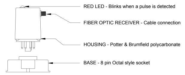
Installation Note: To reduce the chance of noise causing the OPTV-20 to emit false signals, it is recommended that terminal 8 be connected to either panel (earth) ground or terminal 2 on the OPTV-20. Panel ground is the preferred choice of connection.
