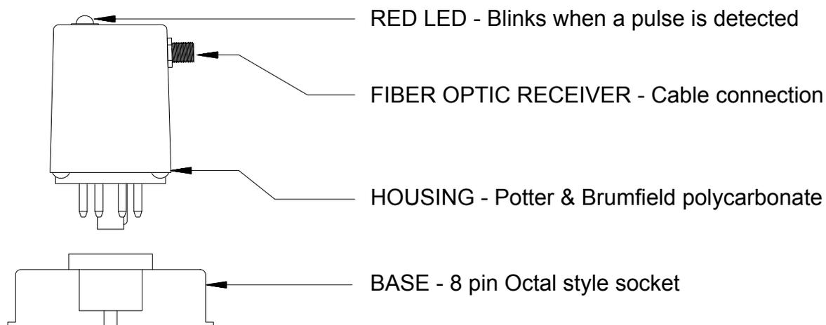
**Installation Note:** To reduce the chance of noise causing the OPTV-20 to emit false signals, it is recommended that terminal 8 be connected to either panel (earth) ground or terminal 2 on the OPTV-20. Panel ground is the preferred choice of connection.
