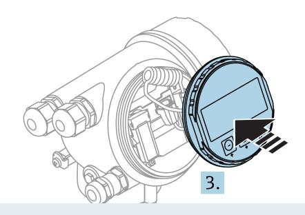
3. Place the display in the upright position. With the Bluetooth module the rotation of the display is not possible.
