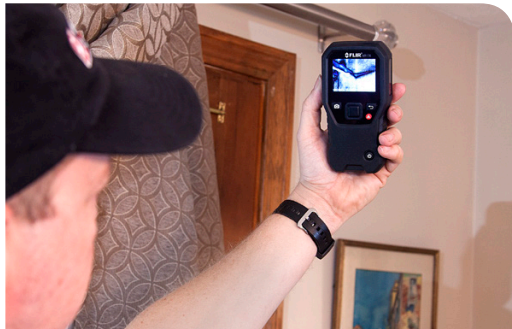
FLIR MR160 scanning ceiling & wall joint for moisture issues.
