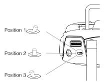
P-mode (Positioning): P-mode works best when the GPS signal is strong. The aircraft utilizes GPS, stereo Vision Systems, and an Infrared Sensing System to stabilize, avoid obstacles or track moving subjects. Advanced features such as TapFly and ActiveTrack are enabled in this mode.
