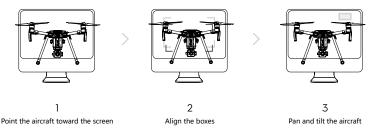
⚠ DO NOT power off or unplug the USB cable after calibration. Wait for data calculation.
