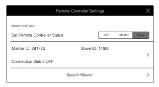
3. Select the Master remote controller from the Master list and input the password to connect.
