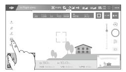
3. Tap on the subject you want to track, then tap to confirm your selection. If the subject is not automatically recognized, drag a box around it. The box \*\* \*\* will turn green when tracking is in progress. If the box turns red, the object was not identified and you should try again.
