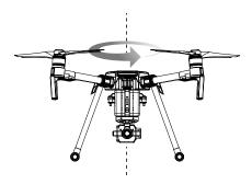
Hold the aircraft vertically, with the nose pointing downward, and rotate it 360 degrees around the center axis. Re-calibrate the aircraft if the aircraft status indicators blink red.
