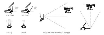
Ensure the aircraft is flying within the optimal transmission zone. To maintain optimal transmission performance, adjust the remote controller and antennas according to the above diagram. The position of the antennas required for optimal transmission range varies in the frequency of 5.8 GHz and 2.4 GHz. Please place the antennas based on the actual operating frequency.
