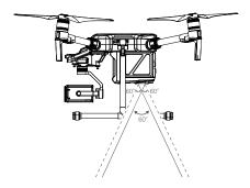
Infrared Sensing System detection range is depicted below.
