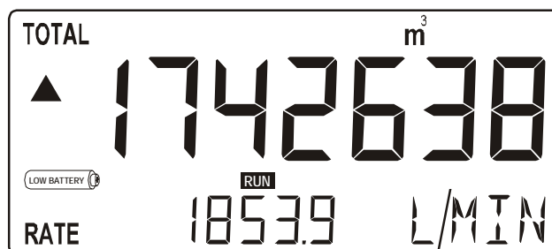
Fig. 4: Example of low-battery alarm.
