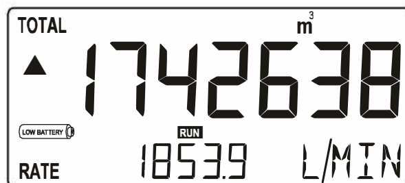
Fig. 4: Example of low-battery alarm.
