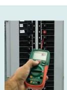
Built-in non-contact IR Thermometer quickly identifies hot spots on electrical panels
