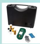
Meter comes complete with all the accessories to conveniently take measurements of both Free and Total Chlorine up to 3.50ppm with 0.01ppm resolution. The method used is adapted from USEPA Method 330.5 for waste water and Standard Method 4500-CI-G for drinking water.
