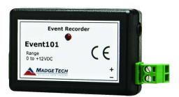
The Event101 records a time-stamped data point when an event takes place within a user defined reading interval. The reading interval can be set using the MadgeTech software to be from one second to twelve hours. When an event occurs on the input of the Event101, the date and time is recorded at the end of the reading interval. By only writing to memory when an actual event occurs on the input, the length of time the loggers can record to memory is maximized (13,107 events).
