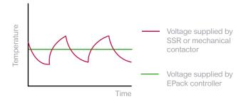
Compared to a standard SSR or mechanical contactor, the EPack Controller adjusts the energy delivered to the heating element, reducing temperature fluctuation and helping to extend the life of the heater.
