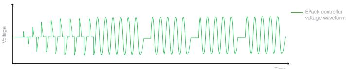
The EPack power controller automatically switches from phase angle to burst firing mode depending upon the ohmic value of the load, for example, during the period of stress when the load is cold. The advanced start-up feature allows smooth start-up with less stress on the load.
