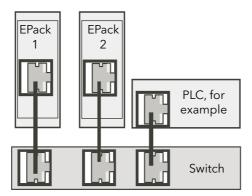
Figure 37 PROFINET Wiring - Multiple controllers
