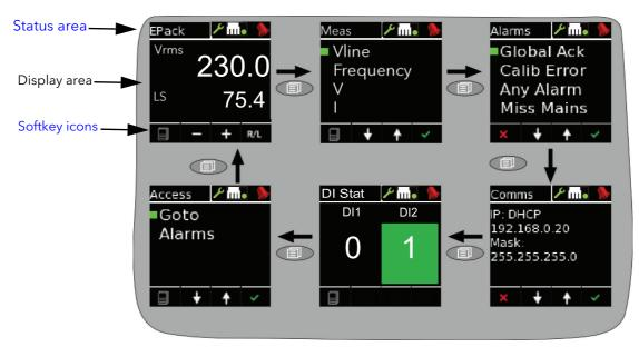
Figure 14 Operator interface
