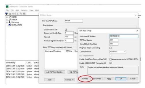
Figure 128 Ethernet Connection Checking using OPC Server
