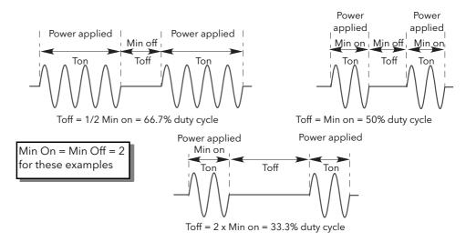
Figure 19 Burst variable firing
