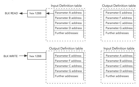
Figure 144 Block read and block write (note 3)
