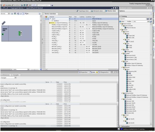
Figure 44 Siemens TIA Portal showing EPack modules and slots
