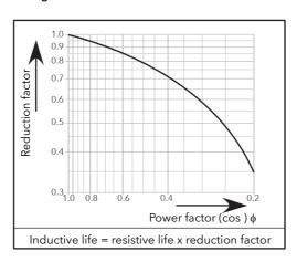
Figure 154 Relay derating curves
