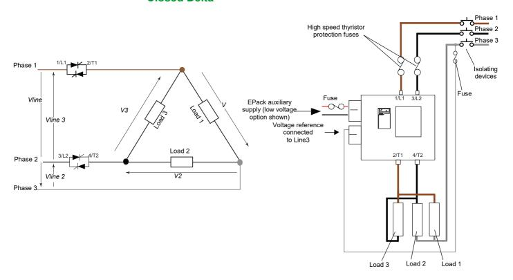
Figure 10 2 phase Closed Delta wiring scheme/load configuration
