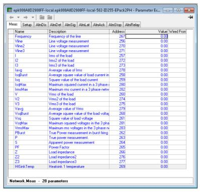
Figure 116 Network, Meas configuration panel
