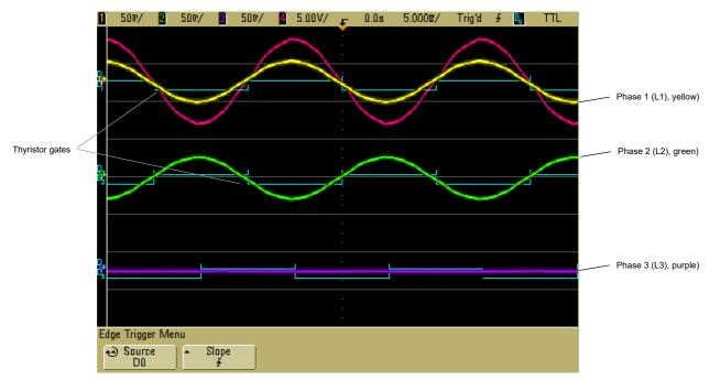
Figure 94 Waveform, unbalanced load (L3 load open circuit), ULM option on, automatically balances thyristor gates and remaining phases 1 and 2.
