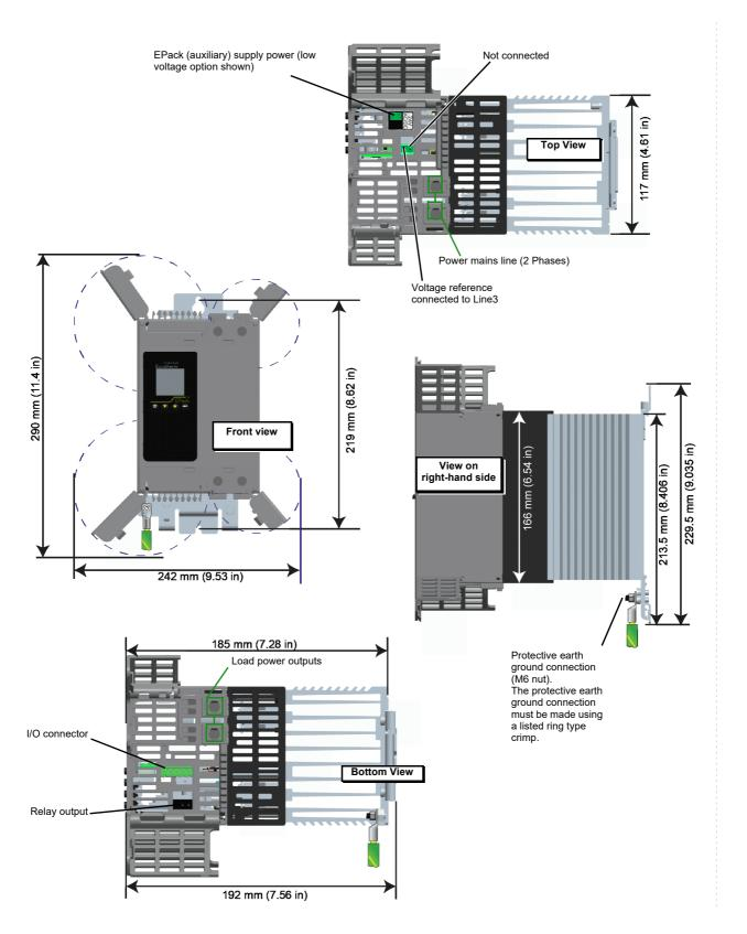
Figure 4 Mechanical installation details (16A to 32A units)
