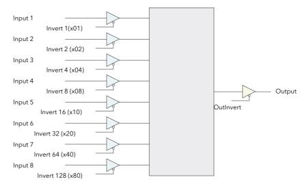
Figure 110 LGC8 Schematic
