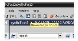
Figure 48 The compiled configuration is downloaded to EPack
