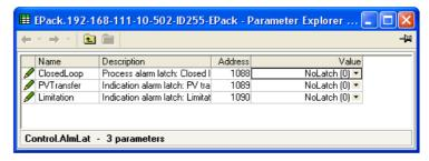
Figure 81 Control Alarm latching page
