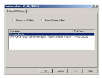
Figure 33 RSLinx Classic configure driver Ethernet/IP settings Now you are in a position to browse your network and locate EPack.
