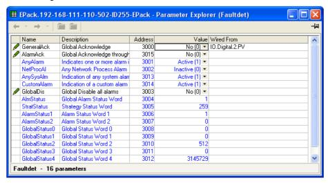
Figure 88 Fault detection menu page
