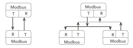
Figure 35 Single Serial Link and Multi Drop Serial Link
