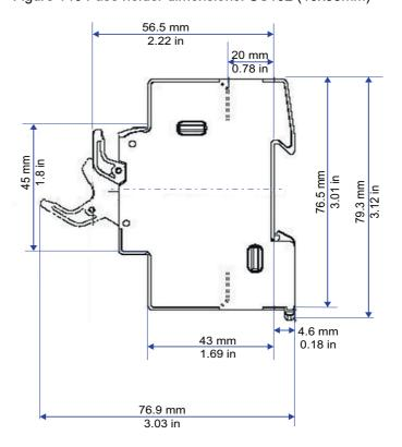
Figure 147 Fuse holder dimensions: CUS102 (10x38mm)
