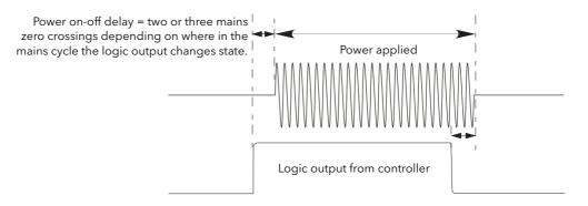
Figure 17 Logic firing mode
