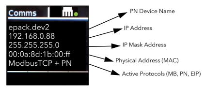
Figure 43 Display of the Device Name on EPack (e.g. "epack.dev2").
