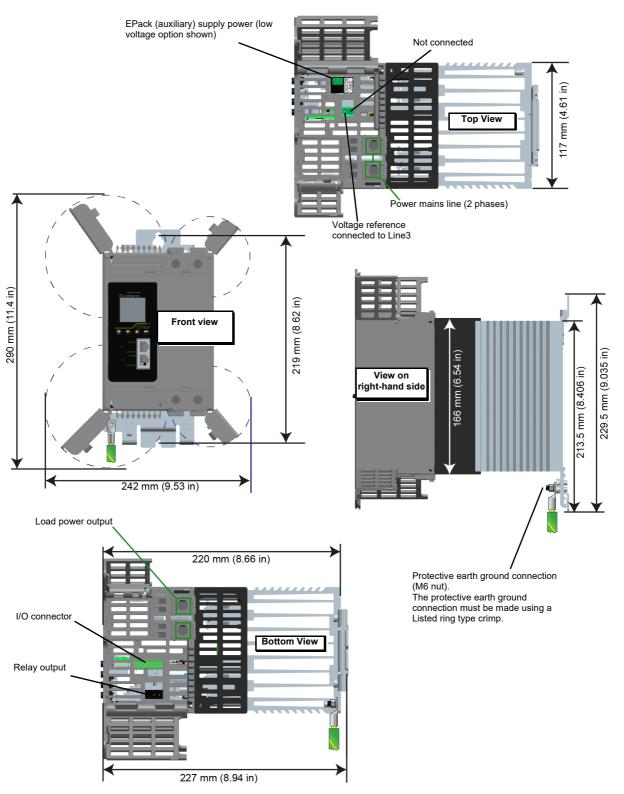
Figure 5 Mechanical installation details (40A to 63A units)
