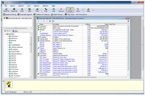
Figure 36 iTools - Ethernet Communications Parameter
