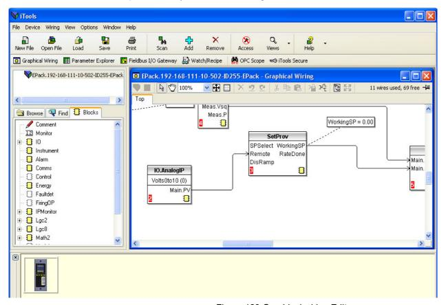
Figure 129 Graphical wiring Editor
