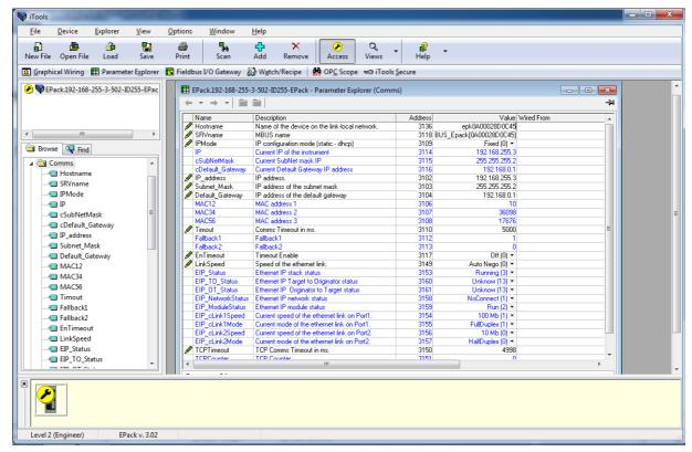
Figure 20 Ethernet/IP User Comms configuration parameters
