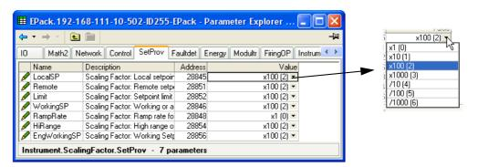
In the above example it can be seen that all the Set point provider parameters are scaled x100, except for Ramp Rate which is not scaled (i.e. the scaling factor = 1). As can also be seen, the scaling factors available are x1, x10, x100, x1000,  $\div$ 100,  $\div$ 1000.
