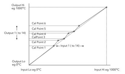
Figure 113 Compensation for Sensor Discontinuities
