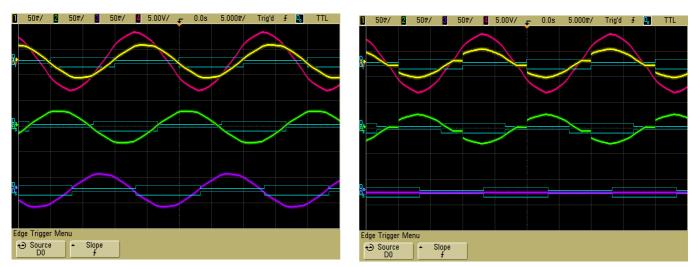
Figure 93 Waveforms; balanced load left, unbalanced load right (ULM off)
