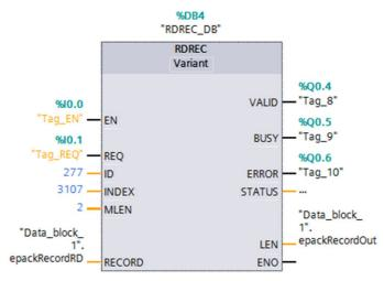
Figure 50 Reading one EPack parameter, using RDREC function block of STEP 7
