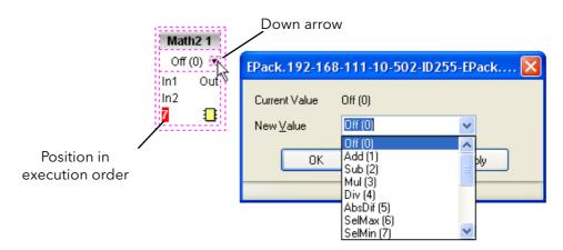
Figure 130 Function block example
