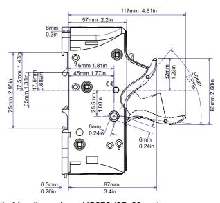
Figure 150 Fuse holder dimensions: US272 (27x60mm)
