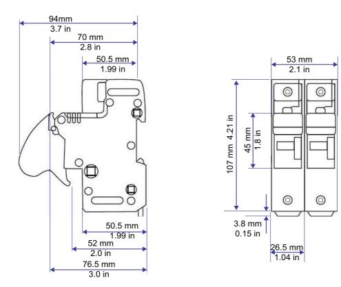
Figure 148 Fuse holder dimensions: US142 (14x51mm)
