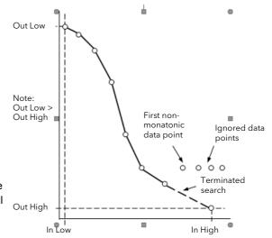
Figure 112 How an Inverted Curve will Terminate its search when it detects non-monatonic data
