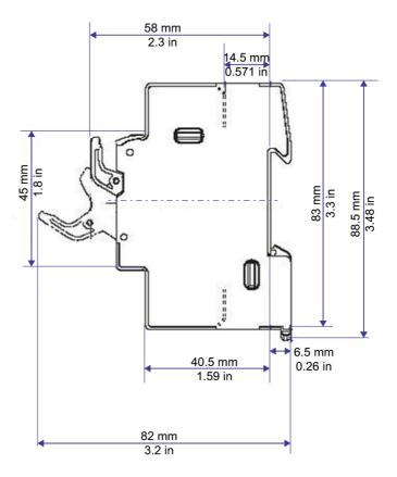
Figure 146 Fuse holder dimensions: US102 (10x38mm)
