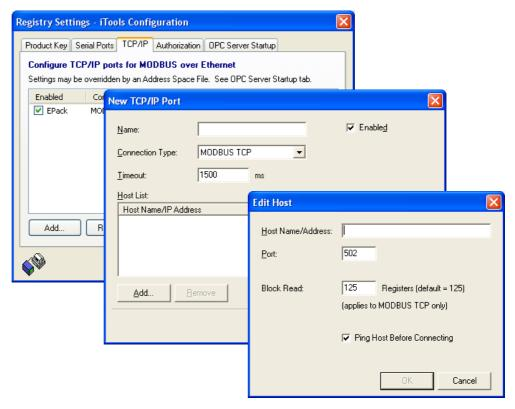
Figure 126 Adding a new Ethernet port
