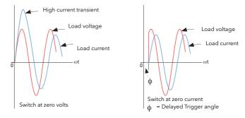
Figure 92 Delayed trigger definition
