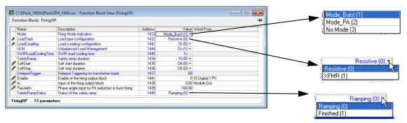
Figure 89 iTools configuration firing output page
