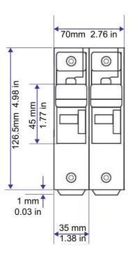
Figure 149 Fuse holder dimensions: US222 (22x58mm)
