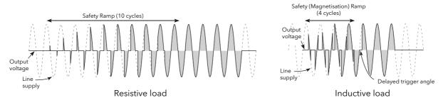
Figure 90 Safety ramp (burst firing) examples
