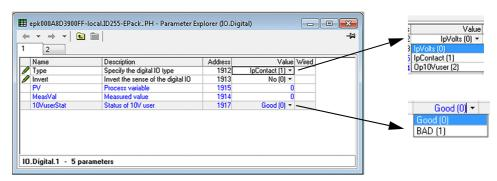
Figure 98 iTools Digital Input configuration page, (digital input 2 displayed)
