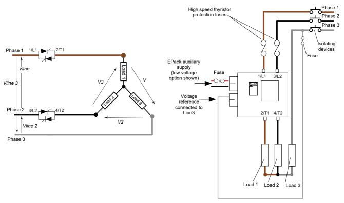
Figure 11 2 phase Star without neutral wiring scheme/load configuration
