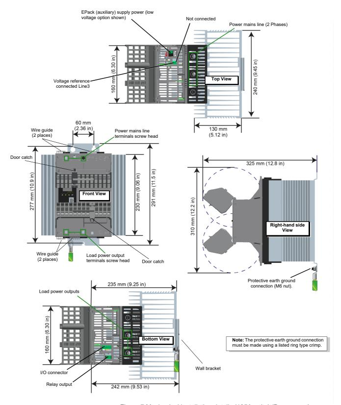
Figure 7 Mechanical installation details (125A units) (Doors open).
