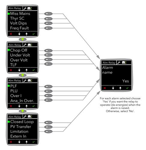
Figure 65 Alarm Relay menu
