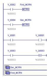
The example at right an MCRN named Sec\_MCRN nested inside the MCRN named First\_MCRN. Whenever the V\_I0002 contact allows power flow into the MCRN function, program execution will continue without power flow to the coils until the associated ENDMCRN is reached. If the V\_I0001 and V\_I0003 contacts are ON, the V\_Q0001 coil is turned OFF and the SET coil V\_Q0003 maintains its current state.
