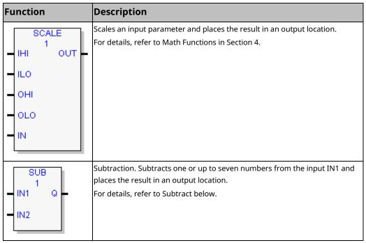
The output is calculated when the instruction is performed without Overflow, unless an invalid operation occurs.
