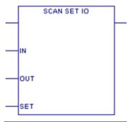
The Scan\_Set\_IO function scans the I/O of a specified scan set number (Modules can be assigned to scan sets in hardware configuration.). You can specify whether the Inputs and/or Outputs of the associated scan set will be scanned.
