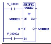
Whenever input V\_I0001 is set, the bits in the input string that begins at WORD1 are copied to the output bit string that starts at WORD2. WORD2 is left-shifted by 8 bits, as specified by the input N. The resulting open bits at the beginning of the output string are set to the value of V\_I0002.
