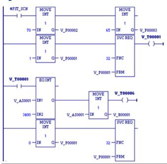
Interrupts from the high-speed counter module whose starting point reference address is %I00065 will be suspended while the CPU solves the logic of the second rung. Without the Suspend, an interrupt from the HSC could occur during execution of the third rung and %T00006 could be set while %R000001 has a value other than 3,400. (%AI00001 is the first non-discrete input reference for the High Speed Counter.)
