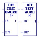
When the Bit Test function receives power flow, it tests a bit within a bit string to determine whether that bit is currently 1 or 0. The result of the test is placed in output Q.
