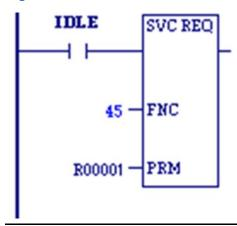
In the following LD example, when the Idle contact passes power flow, the next Output and Input Scan are skipped.
