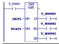
When %I00001 is ON, the integer variable SHIPS is compared with the variable BOATS. Internal coils %M0001, %M0002, and %M0003 are set to the results of the compare.
