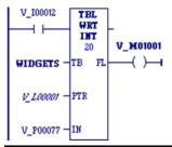
WIDGETS is a table with 20 integer elements. When the enabling input %I00012 is ON, the pointer increments and the contents of %P00077 are written into the table at the pointer location. %L00001 functions as the pointer into the data table.
