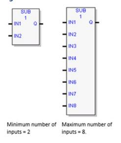
Subtracts the operands IN2 ...IN8 from the operand IN1 and stores the result in the output variable assigned to Q.
