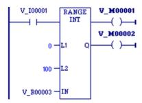
When RANGE\_INT receives power flow from the normally open contact %I0001, it determines whether the value in %R00003 is within the range 0 to 100 inclusively. Output coil %M00002 is ON only if  $0 \le \%$ AI0050  $\le 100$ .
