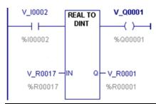
Whenever input %I0002 is set, the REAL value at input location %R0017 is converted to a double precision signed integer (DINT) and the result is placed in location %R0001. The output %Q1001 is set whenever the function executes successfully.
