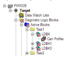
DLBs are created as components of a specific Target and are separate from the application logic block components associated with a target.
