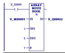
Using bit memory blocks, the input block starts at SR=%M0009, the output block starts at %Q0022, and the length of both blocks is 16 one-bit registers (Length=16).
