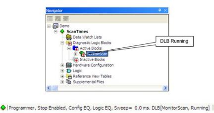
8. Open the DLB block and place the DLB variables in the Data Watch window to observe their operation.
