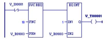
SVC\_REQ reads the status of I/O forced values into location %R1003. If the returned value in %R1003 is 1, there is a forced value, and EQ INT turns the %T0001 coil ON.
