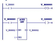
To correct the above problem, the enable input to the ADD instruction should come from a transition (one-shot) coil, as shown below. In the improved circuit, the %I0001 input switch controls a transition coil, %M0001, whose contact turns on the enable input of the ADD function for only one scan each time contact %I00001 closes. For the %M00001 contact to close again, contact %I0001 has to open and close again.
