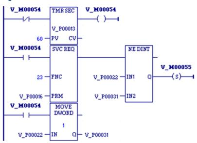
When the timer using registers %P00013 through %P00015 expires, the checksum read is performed. The checksum data returns in registers %P00016 through %P00030. The master program checksum in registers %P00022 and %P00023 (the program checksum is a DWORD data type and occupies two adjacent registers) is compared with the last saved master program checksum. If these are different, coil %M00055 is latched on. The current master program checksum is then saved in registers %P00031 and %P00032.
