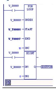
The value for %T00001 (START) is -100 and the value for %T00017 (END) is 100. The INDEX (%R00001) increments by tens, starting at 100 until it reaches it end value of +100. The EQ function of the loop tries to execute 21 times, with the INDEX (%R00001) being equal to 100, -90, -80, -70, -60, -50, -40, -30, -20, -10, 0, 10, 20,
