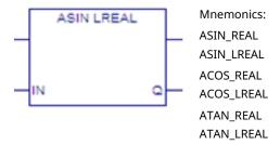
When an Inverse Sine (ASIN), Inverse Cosine (ACOS), or Inverse Tangent (ATAN) function receives power flow, it respectively computes the inverse sine, inverse cosine or inverse tangent of IN and stores the result in radians in output Q.
