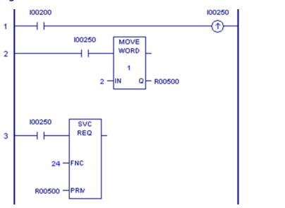
This example resets the module in rack0/slot 2.
