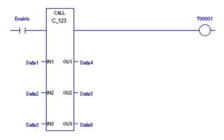
In the example at right, if Enable is set, the C block named C\_123 is executed. C\_123 operates on the input data located at reference addresses Data1, Data2, and Data 3, and produces values located at reference addresses Data4, Data5, and Data6. Logic within C\_123 controls the power flow output.
