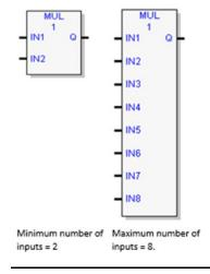
Multiplies two through eight operands (IN1 ... IN8) of the same data type and stores the result in the output variable assigned to Q, also of the same data type.
