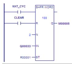
SHFR\_WORD operates on register memory locations %R0001 through %R0100. When the reset reference CLEAR is active, the Shift Register words are set to zero.
