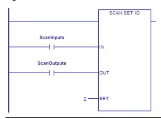
By using the Scan Set IO function block in an interrupt block, you can create a custom I/O scan. For example, two Scan Set IO function blocks can be used in an interrupt block to scan the inputs of a scan set at the beginning of the block and the outputs of the same scan set at the end of the block.
