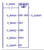
In the example at right, the registers %R0120 through %R0123 are used to store the high and low scaling values. The input value to be scaled is analog input %AI0017. The scaled output data is used to control analog output %AQ0017. The scaling is performed whenever %I0001 is ON.
