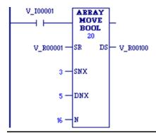
Sixteen (=N) bits that are not byte-aligned are moved from the two 16-bit registers that start at %R00001 (SR) to the two 16-bit registers that begin at %R00100 (DS). For the purposes of this Boolean move, Length is set to 20, because the other 12 bits in either memory block are not considered.
