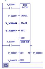
The value for %M00001 (START) is 1 and the value for %M00017 (END) is 10. The INDEX (%R00001) increments by the value of the INC operand (which is assumed to be 1 when omitted) starting at 1 until it reaches the ending value 10. The ADD function of the loop is executed 10 times, adding the current value of I1 (%R00001), which will vary from 1 to 10, to the value of I2 (%R00002).
