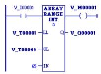
The lower limit (LL) array contains %T00001 through %T00016, %T00017 through %T00032, and %T00033 through %T00048. The lower limit values are 100, 65, and 1. The upper limit (UL) values are 29, 165, and 2. The resulting Q values of 0, 1, and 0 will be placed in %Q00001 through %Q00003. The bit value displayed will be 0 (OFF), representing the value of %Q00001. The power output will be set ON (1).
