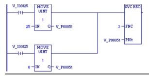
When enabling input %I00125 transitions on, the controller communications window is enabled and assigned a value of 25ms. When the contact transitions off, the window is disabled. The parameter block is in global memory location %P00051.
