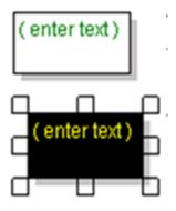
The Text block is used to place an explanation in the program. When you type in a comment, the first few words are displayed.
