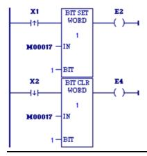
Bit %M00017 is set by a BIT\_SET function and then cleared by a BIT\_CLR function. The positive transition contact X1 activates the BIT\_SET, and the negative transition X2 activates the BIT\_CLR.
