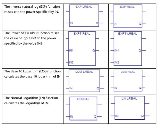
The power flow output is energized when the function is performed, unless or one of the following invalid conditions occurs:
