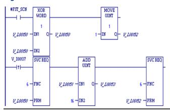
When enabling contact #FST\_SCN is set, the parameter blocks for the checksum task function are built. Later in the program, when input %I00137 transitions on, the number of words being check-summed is read from the CPU operating system. This number is increased by 16, with the results of the ADD\_UINT function being placed in the hold new count for set parameter. The second service request block requests the CPU to set the new word count.
