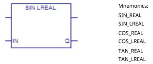
The SIN, COS, and TAN functions are used to find the trigonometric sine, cosine, and tangent, respectively, of an input whose units are radians. When one of these functions receives power flow, it computes the sine (or cosine or tangent) of IN and stores the result in output Q.
