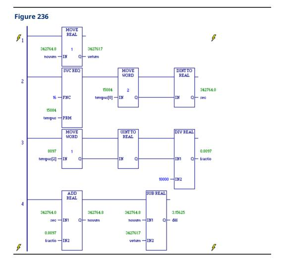
**Note:** Higher resolution (in nanoseconds) can be obtained by using SVC\_REQ 50: Read Elapsed Time Clock.
