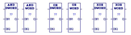
Each scan that power is received, the Logical function examines each bit in bit string IN1 and the corresponding bit in bit string IN2, beginning with the least significant bit in each. You can specify a string length of 1 to 256 WORDs or DWORDs. The IN1 and IN2 bit strings specified may overlap.
