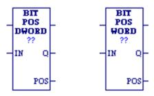
The Bit Position function locates a bit set to 1 in a bit string.
