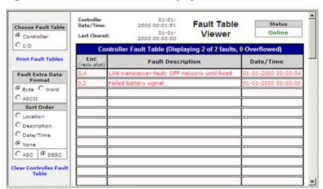
**Figure 261 Controller Fault Table Display**
