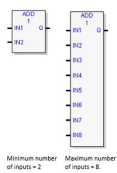
Adds the operands IN1 and IN2 ... IN8 and stores the sum in Q. IN1 ... IN8 and Q must be of the same data type.
