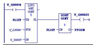
New part numbers (%I00017 - %I00032) are pushed onto a parts array PLIST every time %Q00014 is ON. When the array is filled, it is sorted and the output %Q00025 is turned on. The array PPOSN then contains the original position that the now-sorted elements held before the sort was done on PLIST.
