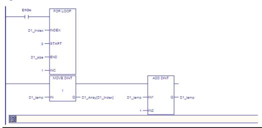
You can use a FOR\_LOOP to iterate through an array's second dimension in a method similar to this example. You can also use nested FOR\_LOOPs to ensure that operations on elements using two variable indexes each do not exceed their array dimension. For additional examples, refer to the online help.
