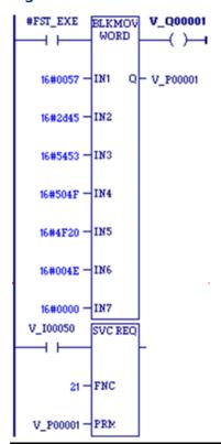
The value passed to IN1 is the fault error code. The value passed in, 16x0057, represents an error code of 87 decimal and will appear as part of the fault message. The values of the next inputs give the ASCII codes for the text of the error message.
