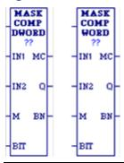
The Masked Compare (MASK\_COMP\_DWORD and MASK\_COMP\_WORD) function compares the contents of two-bit strings. It provides the ability to mask selected bits.
