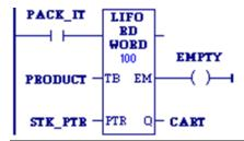
PRODUCT is a LIFO table with 100 word-sized elements. When the enabling input PACK\_IT is ON, the data item at the top of the table is copied into the reference indicated by the nickname CART. The reference identified by STK\_PTR contains the table pointer. Output coil EMPTY indicates when the table is empty.
