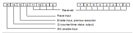
**Note:** Bits 0 through 13 are not used for counters.
