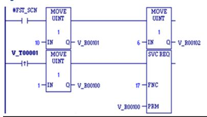
When %T00001 transitions on, alarm interrupts from input %AI0006 are masked. The parameter block at %R00100 is set up on the first scan.
