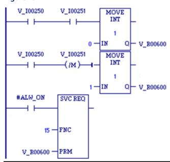
When inputs %I0250 and %I0251 are both on, the first Move function places a zero (read Controller Fault Table) into the parameter block for SVC\_REQ 15. When input %I0250 is on and input %I0251 is off, the Move instruction instead places a one (read I/O Fault Table) in the SVC\_REQ parameter block. The parameter block is located at location %R0600.
