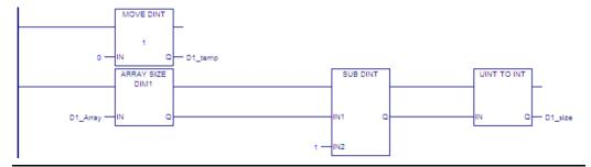
In the following rungs, the FOR\_LOOP executes when D1ON is set to On. The variable index D1\_Index increments by 1 from 0 through D1\_size, the value calculated by ARRAY\_SIZE\_DIM1 and SUB\_DINT. In each loop, the value of D1\_temp is assigned to the element D1\_Array[D1\_Index] and D1\_temp is increased by 1.
