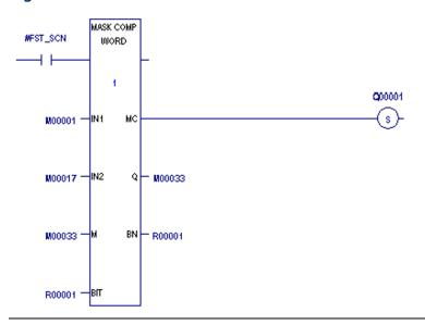
On the first scan, the Masked Compare Word function executes. %M0001 through %M0016 is compared with %M0017 through %M0032. %M0033 through %M0048 contains the mask value. The value in %R0001 determines the bit position in the two input strings where the comparison starts.
