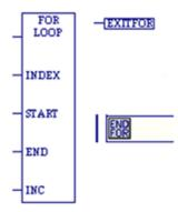
A FOR loop repeats rung logic a specified number of times while varying the value of the INDEX variable in the loop.
