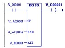
Because a reference is entered for ALT, the values at %AQ001—004 are not written to output modules. When DO\_IO receives power flow, the PLC writes the values from references %R0001-0004 to the analog output modules and %Q0001 is turned on.
