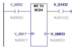
Whenever input %I0002 is set and no errors exist, the INT values at input locations %I0017 through %I0032 are converted to four BCD digits, and the result is stored in memory locations %Q0033 through %Q0048. Coil %Q1432 is used to check for successful conversion.
