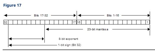
Register use by a single floating-point number is diagrammed below. For example, if the floating-point number occupies registers R5 and R6, R5 is the least significant register and R6 is the most significant register.
