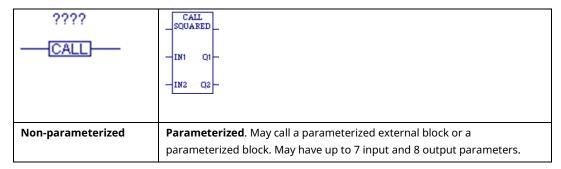
When the CALL function receives power flow, it causes the logic execution to go immediately to the designated program block, external C block (parameterized or not), or parameterized block and execute it. After the block's execution is complete, control returns to the point in the logic immediately following the CALL instruction.
