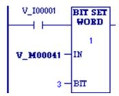
Whenever V\_I00001 is set, %M00043, the third bit of the string beginning at %M00041, is set to 1. Note that neither the status nor the transition value of any of the other bits in the same byte as %M00043 (e.g., %M00041, %M00042, %M00044, etc.) is affected by the BIT\_SET function
