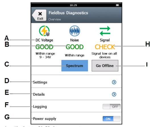
Figure 5-2: Fieldbus Diagnostics Overview screen while taking measurements
