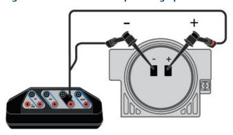
Figure 4-16: Connection for powering a positioner
