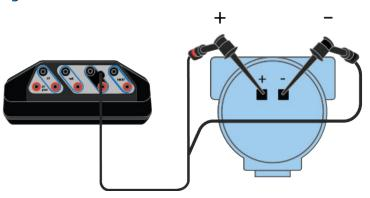
Figure 3-30: Power a HART positioner
