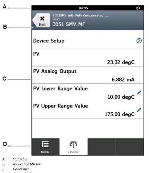
Figure 3-4: Sections of a device screen
