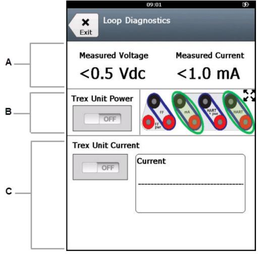
Figure 4-1: Loop Diagnostics screen at start up
