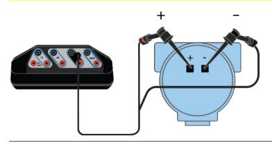
Figure 4-5: Measure voltage on an externally-powered HART transmitter
