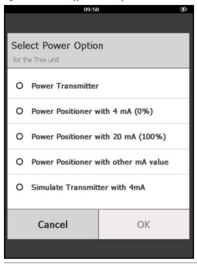
Figure 4-3: Select the type of device to power
