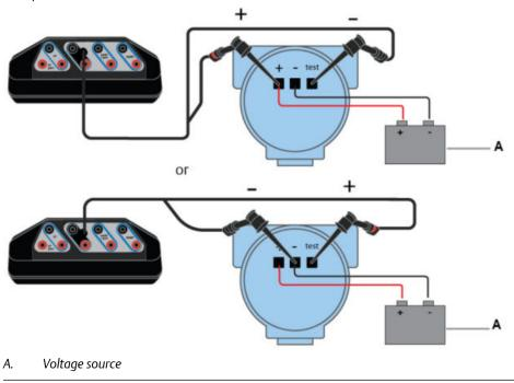
Figure 4-13: Power and control current to simulate a transmitter on an unpowered loop
