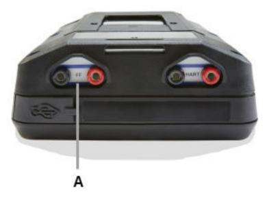
A. FF terminals to communicate with a FOUNDATION fieldbus device
