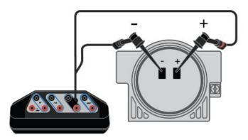
Figure 4-7: Connect to an externally-powered positioner in-parallel
