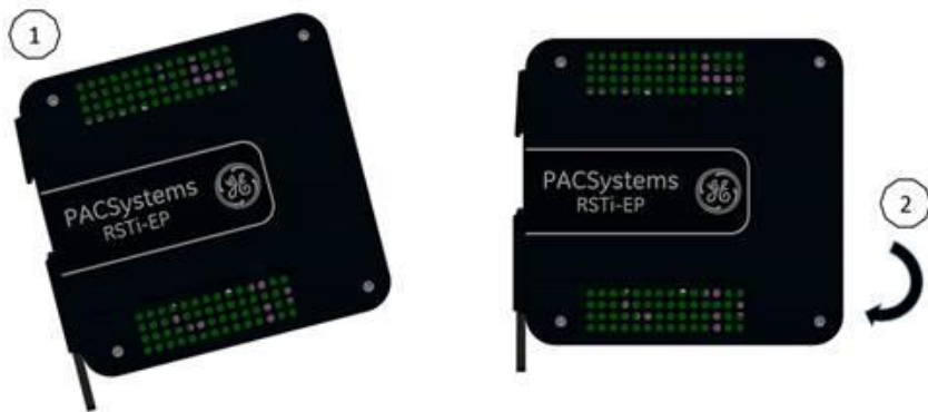
Figure 3: Mounting positions of the EPSCPE100 on DIN rail
