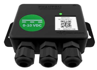
With the General Purpose Phantom you can adapt the data collection to your specific needs. Take **any 0-10V sensor** and make it wireless.
