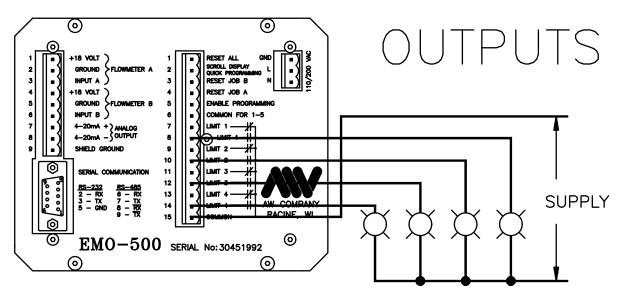
FOR LOAD FROM 1 TO 5 AMP. MAXIMUM LOAD PER OUTPUT: USE OUR RHN SERIES RELAYS INDUCTIVE: DC:10W - AC:20V
