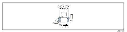
Order code for "Design", option C "Insertion length short ISO/DVGW until DN300, w/o inlet and outlet runs, constricted meas.tube"
