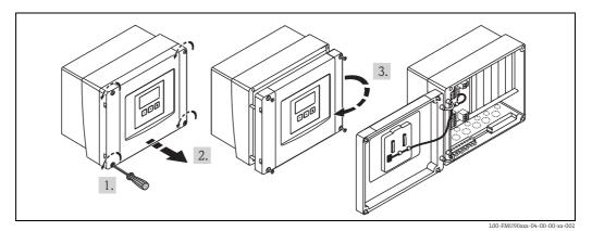
For easier wiring, the lid can be completely removed by unplugging the display plug and loosening the hinges:
