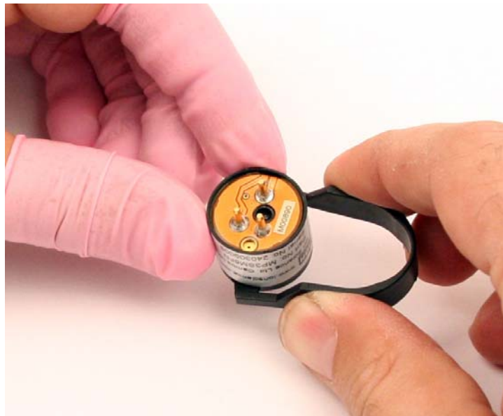
Figure 29: Using Removal Tool
