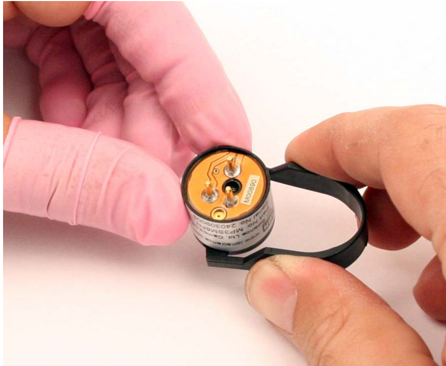
Figure 35: Using Removal Tool
