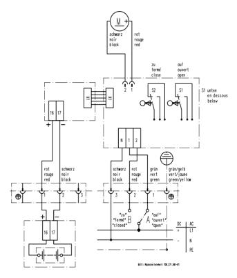
The fail-safe return unit is mounted on the base board and is connected electrically via a flat cable. If the supply voltage is interrupted, the electronics will switch to the storage battery automatically after 5 sec. With a touch control, the function «Go to the CLOSED or OPEN position» can be selected. **Position 1/2: CLOSED, position ON: OPEN** (always both, see at left). The storage battery is charged continuously. Full recharging takes approximately 15 hours.
