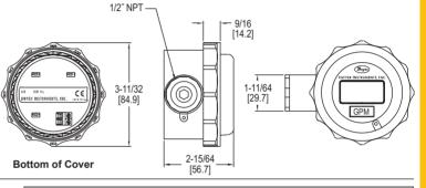
The MODEL LPI Micro-Pressure Based Loop Powered Indicator accepts a 4-20 mA input signal and displays the associated process variable such as pressure, level, flow, temperature, or relative humidity. The indicator is housed in a NEMA 4X (IP66) polycarbonate enclosure with a 1/2" female NPT side port. Users can quickly modify the instrument configuration via three push buttons on the front of the unit.
