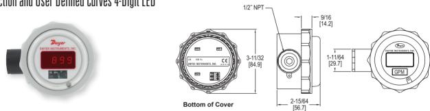
The **MODEL LPI** Micro-Pressure Based Loop Powered Indicator accepts a 4-20 mA input signal and displays the associated process variable such as pressure, level, flow, temperature, or relative humidity. The indicator is housed in a NEMA 4X (IP66) polycarbonate enclosure with a 1/2" female NPT side port. Users can quickly modify the instrument configuration via three push buttons on the front of the unit.
