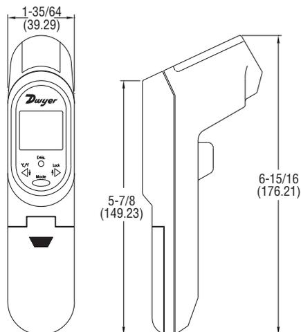
The Series IR3 Infrared Thermometer utilizes infrared technology for precise, non-contact temperature measurement. Models feature a 12:1 distance to target ratio and single point laser sighting for accurate temperature measurements. The IR3 offers an adjustable emissivity, backlit display, selectable temperature units, high/low alarms, minimum, maximum, differential and average functions.
