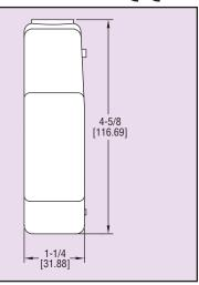
The Model DDM-01 Laser Distance Meter offers quick measurement of distances up to 229.7 feet (70 meters) with the click of a button. It is also able to easily make area and space calculations and volume measurements from what it records. Another feature of the Model DDM-01 is that it is able to use the Pythagorean Theorem to indirectly calculate the height of an object. The meter can read out in feet, inches, or meters and includes a backlight for use in dark areas.
