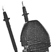
Fig. 3: Utilize rubber test lead holster
