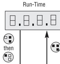
If no buttons are pressed for a minute or more, the device assumes run-time mode. The display shows the PV (if the input is in range) or shows **----** or **----** to indicate over/under range. In order to access menu configuration mode, the user must press **ENTER** followed immediately by **CYCLE**. In order to exit the menu and return to run-time, a user must press **ESCAPE**.
