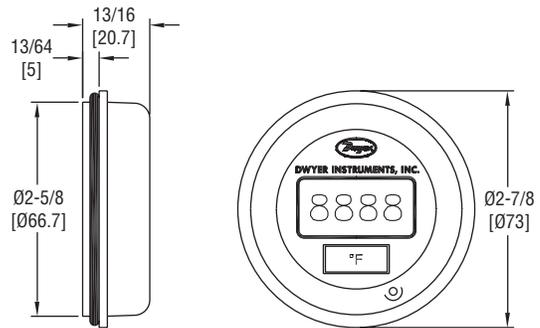
The **Series BPI** is a range of battery powered temperature indicators. The Series BPI-XX1 accepts an RTD sensor; the Series BPI-XX2 accepts a thermocouple sensor. The sensor type, temperature units and other flexible configuration settings are selectable via a simple to use menu system, which is navigated by the use of three push-button keys located on the rear of the display. The entire assembly is sealed into a cap that fits directly onto the connecting heads.
