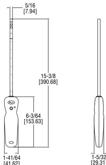
The Model AP2 Wireless Thermo-Anemometer Probe measures air velocity, air flow, and temperature when combined with the Model UHH Universal Handheld. In order to prevent damage to the sensing element, the probe has a protective sleeve that slides over the sensor when it is not in use. Markings on the probe allow users to know the insertion depth to obtain better accuracy when traversing the duct.
