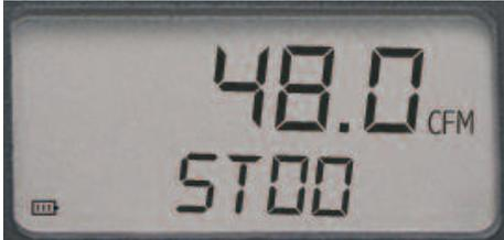
From the home screen, push **MEMORY/UP** to view all previously stored values. Cycle up or down through the stored data with the **MEMORY/UP** or **STORE/DOWN** buttons. From the home screen, press **STORE/DOWN** to store data points to memory. For both data storage and data memory retrieval, press **MENU** to return to the home screen.
