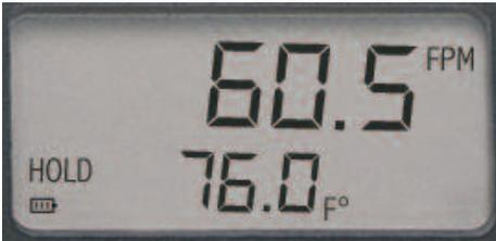
HOLD will appear on the home screen when the **HOLD** button is pressed, indicating the process reading has been frozen.
