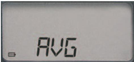
Press **ENTER** to view the AVG function. This function will adjust the process reading on the home screen to report the average reading over the period of selected time. Press **MEMORY/UP** or **STORE/DOWN** to select between 0, 10, 30, or 60 second values. Push **ENTER** to store the desired value.
