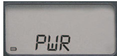
Push **ENTER** to see current time off setting. Select 30 or 10 values indicating minutes for power to automatically shut-off. By selecting 0, the auto shut-off is disengaged and the unit will only turn off manually by the **ON/OFF/LIGHT** button.
