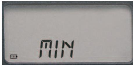
Push **ENTER** to see the minimum recorded reading. When viewing the minimum recorded reading, hold **ENTER** for 4 seconds to clear. Push **MEMORY/UP** or **STORE/DOWN** to cycle through parameters.
