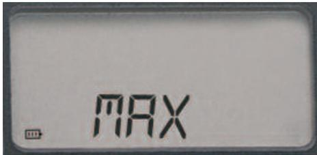
Push **ENTER** to see the maximum recorded reading. When viewing the maximum recorded reading, hold **ENTER** for 4 seconds to clear. Push **MEMORY/UP** or **STORE/DOWN** to cycle through parameters.
