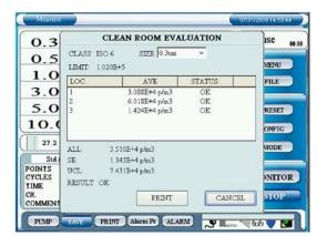
3905 ISO mode results showing UCL and passing results for a Class 6 cleanroom
