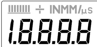
The numeric portion of the display consists of 4 complete digits preceded by a leading "1", and is used to display numeric values, as well as occasional simple words, to indicate the status of various settings. When the **MMX-6 DL** is displaying thickness measurements, the display will hold the last value measured, until a new measurement is made. Additionally, when the battery voltage is low, the entire display will begin to flash. When this occurs, the batteries should be replaced.
