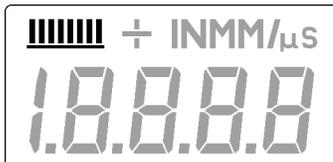
These eight vertical bars form the Stability Indicator. When the **MMX-6 DL** is idle, only the left-most bar and the underline will be on. While the gauge is taking a measurement, six or seven of the bars should be on. If fewer than five bars are on, the **MMX-6 DL** is having difficulty achieving a stable measurement, and the thickness value displayed will most likely be erroneous.
