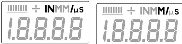
When the **IN** symbol is on, in conjunction with the **/μs** symbol, the **MMX-6 DL** is displaying a sound-velocity value in **inches-per-microsecond**.
