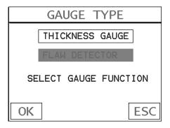
Power up the **DFX-8**, by pressing the on/off key located in the bottom right corner of the keypad. During initial boot up, a flash screen and lights will be displayed, followed by a **GAUGE TYPE** selection screen. Since this manual will focus on the thickness gauge portion of the **DFX-8**, use the **UP/DOWN** arrow keys to select "thickness gauge", followed by pressing the **OK** key start the **DFX-8** in thickness mode.
