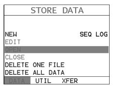
2) Use the **UP** and **DOWN** arrow keys on the left button wheel to scroll through the sub menu items until **OPEN** is highlighted.
