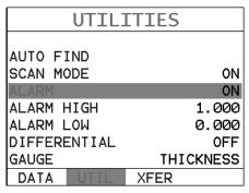
1) Press the **MENU** key once to activate the menu items tab. Press the **MENU** key multiple times to tab right, and the **ESC** key multiple times to tab left, until the **UTIL** menu is highlighted and displaying the submenu items.
