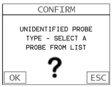
1) Press the **OK** or **ESC** keys to display the factory list of transducer types (by diameter and frequency).
