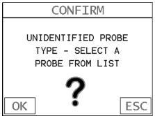
5) Press the **OK** or **ESC** keys to display the factory list of transducer types (by diameter and frequency).
