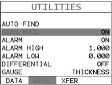
1) Press the **MENU** key once to activate the menu items tab. Press the **MENU** key multiple times to tab right and the **ESC** key multiple times to tab left until the **UTIL** menu is highlighted and displaying the submenu items.
