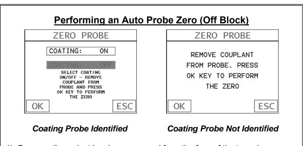
1) Be sure all couplant has been removed from the face of the transducer.
