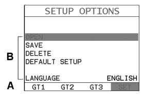
1) Press the **MENU** key once to activate the menu items tab. Press the **MENU** key multiple times to tab right, and the **ESC** key multiple times to tab left until the desired tab group is highlighted and displaying the submenu items. Alternatively, press the **LEFT** and **RIGHT** arrow keys multiple times using the left button wheel. The tab groups are illustrated above (A).
