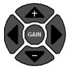
1) Press the GAIN key once to display the Digits Edit Box. Press the MENU key multiple times to tab right, and the ESC key multiple times to tab left, until the TUNE menu is highlighted and displaying the submenu items. Alternatively, press the LEFT and RIGHT arrow keys multiple times using the left button wheel.
