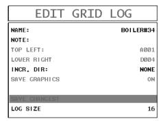
10)Press the **UP** or **DOWN** arrow key to highlight **SAVE CHANGES**, and the **OK** key to activate the confirmation screen.
