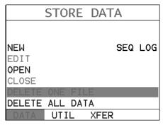
3) Press the **ENTER** key to close the active file. **Note:** Following the key press, the **CLOSE** text will be grayed out indicating the file has been closed and is no longer active.
