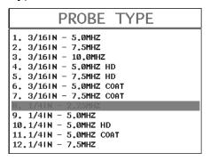
6) Press the **UP** and **DOWN** arrow keys on the left button wheel to scroll through the transducer list until the appropriate type is highlighted.
