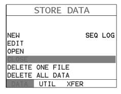
2) Use the **UP** and **DOWN** arrow keys on the left button wheel to scroll through the sub menu items until **CLOSE** is highlighted.
