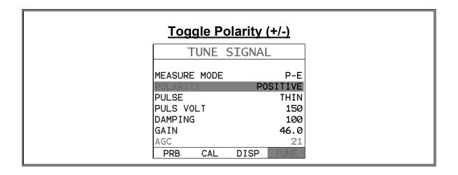
**Note:** Before toggling the **Polarity**, the **DFX-8** should be set to the **RF** display view option. The **RF** view will give the user the best opportunity to correctly view the positive and negative cycles of the waveform. Please refer to page 64 for information on selecting the **Display Views**.
