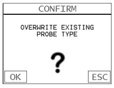
3) Press the **ENTER** key to select the transducer type and display overwrite existing probe screen.
