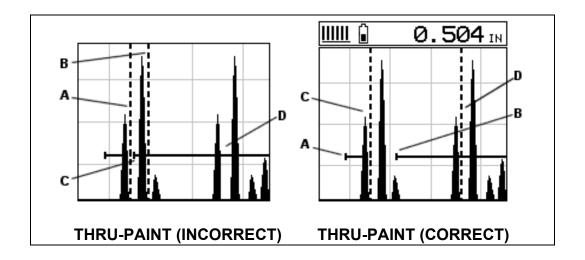
Refer to the incorrect diagram above. Point **(A)** represents the detection on the first back wall echo. The true, second back wall, reflection should be detecting at point **(D)**. However, the hold-off **(C)** is setup incorrectly and the **DFX-8** is detecting the ring down noise of the transducer, on the first reflection, rather than the true second back wall reflection shown at **(D)**.
