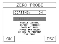
3) Press the **UP** and **DOWN** arrow keys on the left button wheel to toggle the coating option on/off.
