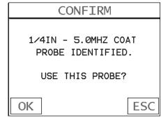
1) Press the **OK** key once to use the identified probe, or **ESC** to display a list of optional transducers. *Note: if the* **DFX-8** recognizes a specific transducer, the user should always select **OK** to use the identified probe. The only time
