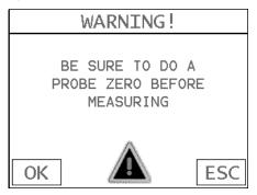
**Note:** When the zero probe option is set to manual, the probe zero disk (battery cap) located on the top of the gauge will be used as a zero standard and the warning screen illustrated above will be displayed.
