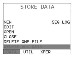
2) Use the UP and DOWN arrow keys on the left button wheel to scroll through the sub menu items until DELETE ALL DATA is highlighted.
