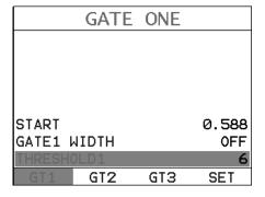
1) Press the **MENU** key once to activate the menu items tab. Press the **MENU** key multiple times to tab right, and the **ESC** key multiple times to tab left, until the **GT1** menu is highlighted and displaying the submenu items.
