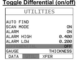
Press the MENU key once to activate the menu items tab. Press the MENU key multiple times to tab right, and the ESC key multiple times to tab left, until the UTIL menu is highlighted and displaying the submenu items.
