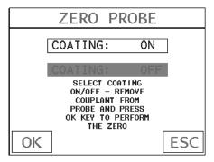
3) Press the **UP** and **DOWN** arrow keys using the left button wheel to toggle the coating option on/off.
