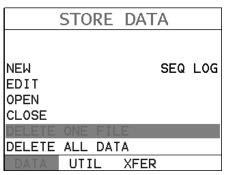
2) Use the **UP** and **DOWN** arrow keys on the left button wheel to scroll through the sub menu items until **DELETE ONE FILE** is highlighted.
