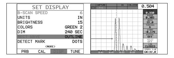
**Filled** – Draws a filled version of the waveform.
