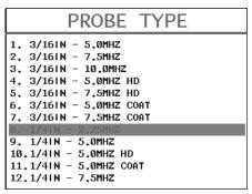
2) Press the **UP** and **DOWN** arrow keys on the left button wheel to scroll through the transducer list until the appropriate type is highlighted.
