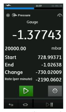
Figure 2-27 Leak Test Example
