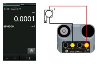
Figure 2-20 Measure current on CH1. Range ±55 mA
