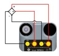
Figure 2-25 Measure DC Volts (10V) or DC mV (10V) on CH1
