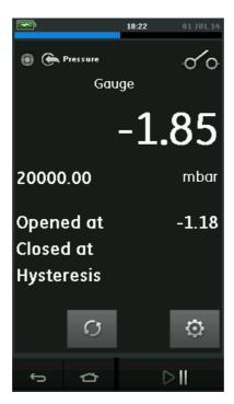
Figure 2-15 Switch Test Example
