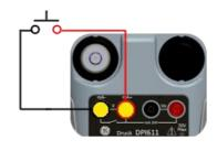
Figure 2-24 Switch Test
