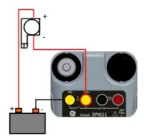
Figure 2-22 Measure current with external loop power (Range: ±55mA)
