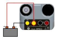
Figure 2-21 Measure DC Volts or DC mV on CH1.
