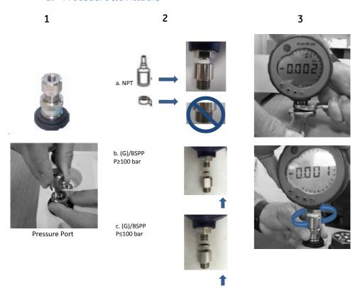
Figure 2-2 Attach / Remove Pressure connections
