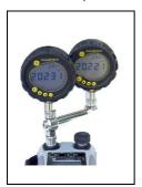
For greater efficiency, two test devices can be connected at the same time. The adaptor connects to the pressure port of the DPI612 and provides two outlet ports. It is compatible with the standard adaptors supplied and the adaptor kits.
