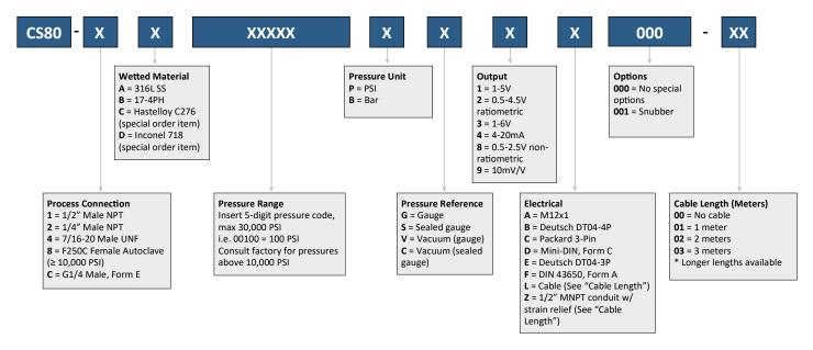
Ordering Example: CS80-1A00200PG4A000-00 (1/2" Male NPT, 316L SS, 0-200 PSI gauge, 4-20mA, M12x1)
