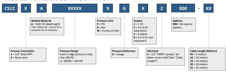
Ordering Example: CS12-6A00005PG4Z000-10 (Nose cone, 316L SS, 0-5 PSI gauge, 4-20mA, 1/2" MNPT conduit with nylon strain relief, 10 meters of ETFE cable) Not all configurations are available. Our sales team can recommend the closest available configuration based on your requirements. Contact Core Sensors for configurations not shown.
