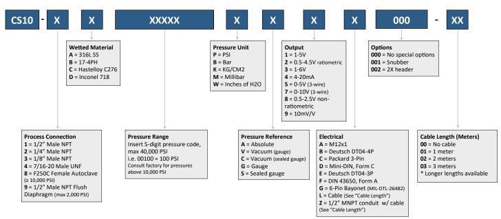
Ordering Example: CS10-2A01000PS4A000-00 (1/4" Male NPT, 316L SS, 0-1000 PSI sealed gauge, 4-20mA, M12x1)
