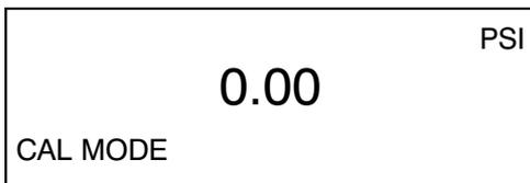
Use the Pressure Standard to output 0.00 psi. After the output has stabilized, press the ENTER key to continue. As the unit takes readings, the screen will show \_\_\_\_\_. When the readings are complete the screen should look as shown below.
