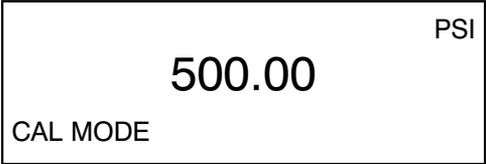
Use the Pressure Standard to output 500.00 psi (100%). After the output has stabilized, press the ENTER key to continue. As the unit takes readings, the screen will show \_\_\_\_\_. When the readings are complete the screen should look as shown in the illustration that follows.
