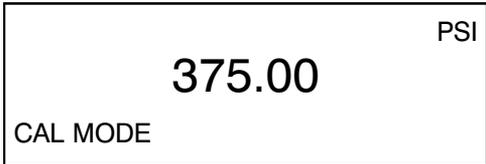
Use the Pressure Standard to output 375.00 psi (75%). After the output has stabilized, press the ENTER key to continue. As the unit takes readings, the screen will show \_\_\_\_\_. When the readings are complete the screen should look as shown below.
