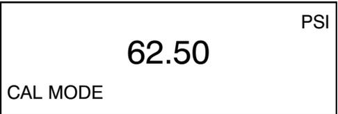
Use the Pressure Standard to output 62.50 psi (12.5%). After the output has stabilized, press the ENTER key to continue. As the unit takes readings, the screen will show \_\_\_\_\_. When the readings are complete the screen should look as shown below.
