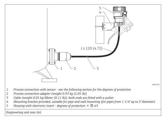
Degree of protection for the process connection and sensor with the use of
