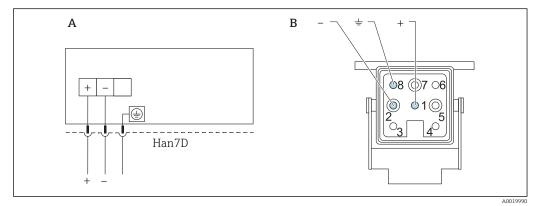
Electrical connection for devices with Harting plug Han7D Α
