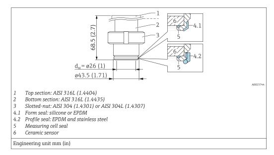
The roughness of the surface in contact with the medium is  $R_a$  < 0.76  $\mu m$  (30  $\mu in).$
