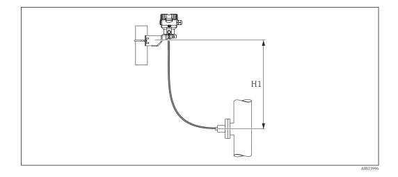
The maximum height difference depends on the density of the filling oil and the smallest ever pressure that is permitted to occur at the diaphragm seal (empty vessel), see illustration below. The following diagram depicts the maximum installation height above the lower diaphragm seal for vacuum applications.
