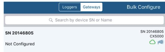
If the gateway does not appear, make sure it is powered up and within range of your phone or tablet or press the button on the gateway.
