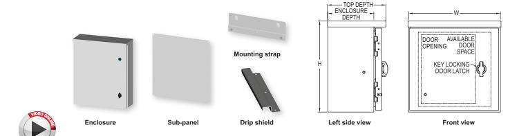
The Series CSE-3R Galvannealed Steel Enclosures are spot-welded, wall mounted enclosures designed to house electrical controls, instruments, and components in an outdoor environment. These units are made of carbon steel, NEMA 3R outdoor environment rated and carry a UL approval.
