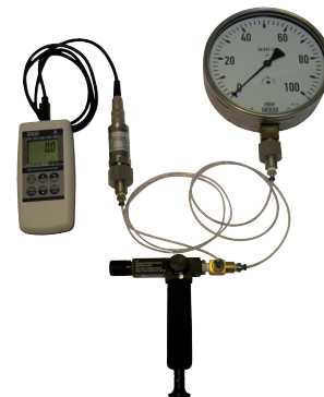
Application, calibration with model CPP7 hand test pump and model CPH6200 reference measuring instrument
