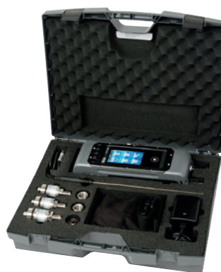
Service case with process calibrator and accessories
