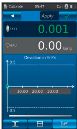
Representation of calibration results as graph
