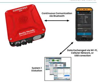
The COMMTEST portable connects via Bluetooth to the handheld, which you can then sync with System 1.
