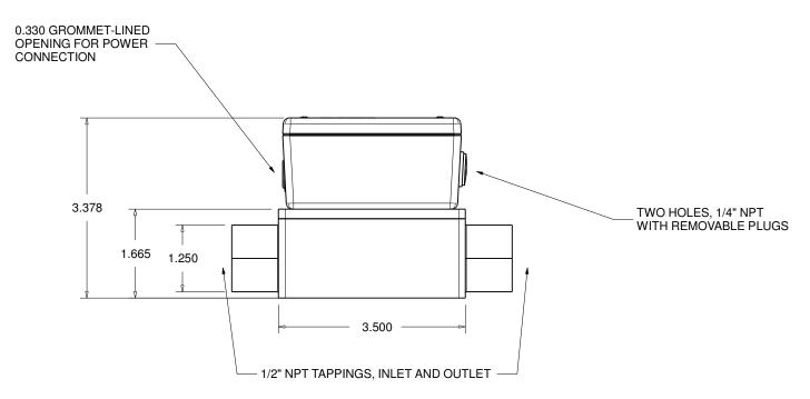
NOTE: 6" LG. X 1/2" DIA. PIPE INCLUDED WITH THE METER, WHICH MUST BE THREADED INTO THE UPSTREAM TAPPING IN THE ALUMINUM BLOCK
