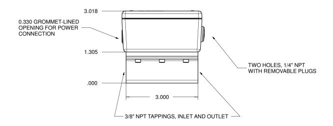
NOTE: 6" LG. X 3/8" DIA. PIPE INCLUDED WITH THE METER, WHICH MUST BE THREADED INTO THE UPSTREAM TAPPING IN THE ALUMINUM BLOCK
