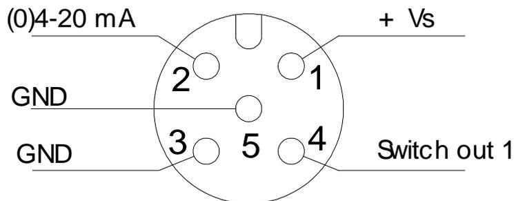
Terminals 3 and 5 are linked internally and can therefore be used either for the output signal or the power supply.
