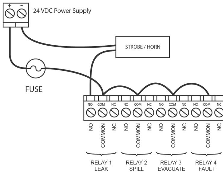
Figure 2-10. Typical DC External Alarm Relay 1 Wiring
