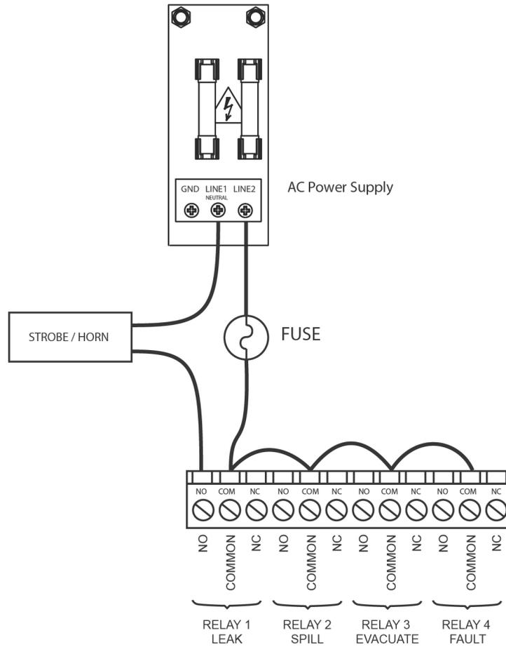
Figure 2-9. Typical AC External Alarm Relay 1 Wiring
