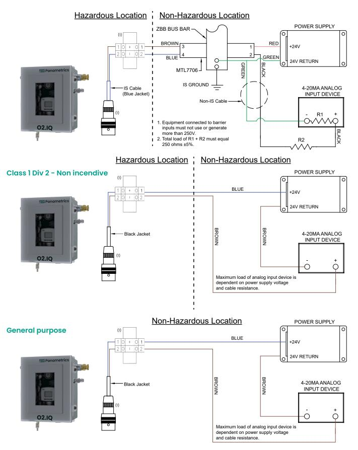
Note: Wiring to integrated terminal strip to be completed at installation site. oxy.IQ connection cable ships separately.
