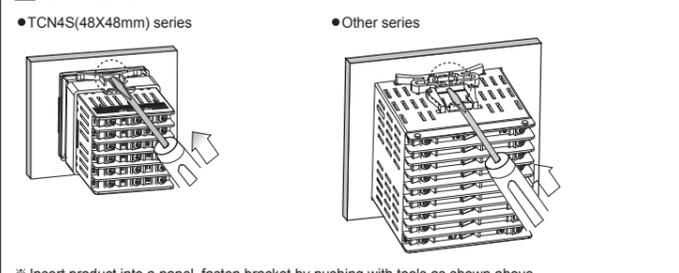
※ Insert product into a panel, fasten bracket by pushing with tools as shown above.
