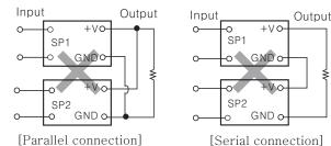
\*\*The power supply shouldn't be used in serial and parallel connection in any case. Please use it individually always.
