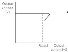
•It is able to protect overcurrent by load with built in overcurrent protection circuit. When the over rated current is flowed, the circuit is operated (Output voltage is fallen.) and it is released when the load current is under the rated current.
