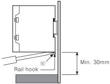
\*When mounting the power supply on the rail, place the item at least 30mm above from the floor to remove easily.
